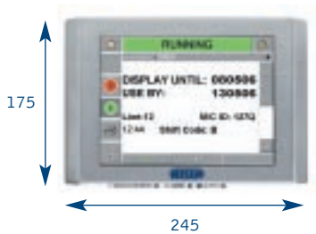
Controller Front Elevation
